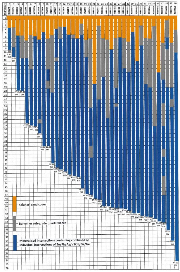
Nxuu Deposit Ga/Ge/V2O5 Mineralisation together with Zn/Pb/Ag Mineralisation
